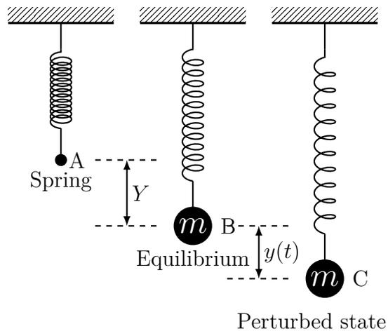
$Y$  is the elongation of the spring in the downward direction caused by the mass  $m$ .  $y(t)$  is the distance traveled by the mass from the equilibrium position. The spring constant is  $k$ . If we do not know the value of  $k$  we can solve for it. From physics we know that the force of the spring is nearly proportional to  $Y$ . So at equilibrium we can write the following equations to solve for  $k$ :
